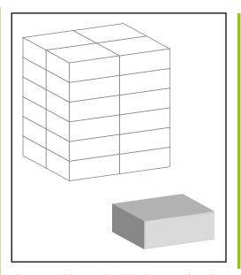
Pieces per package: 1000 Internal protection: BAGS INTENDED TO COME INTO CONTACT  $\mathsf{Packaging:} \underline{10X100} \underline{=} \underline{10}00$ Box length (cm): 40 Box width (cm): 34 Box height (cm): 24,5Gross weight (Kg): 1,5Boxes on a pallet: 48 External protection: <u>STRETCH FILM AND PROTECTION COVER</u>
